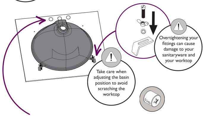
Mark your tap holes leaving space for your taps to be connected without obstructing the basin. A mixer tap (one hole) requires a 35mm hole, Basin taps (2 holes) require 30mm holes and 3H basin taps (3 holes) require centre hole to be 35mm and the two outside holes to be 30mm.
