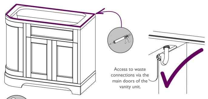
Carefully place the worktop on the unit and secure in place. Once the worktop is in the correct position, apply silicone sealant along the back of the worktop. This will prevent any water from getting behind the unit. Wipe any excess silicone sealant with a soft cloth. Refer to tap/waste
