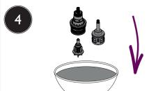
Remove any O-rings and soak all components in de-scaler and wash off in clean water. Examine all seals and replace if needed. Use a WRAS approved silicon based grease on all seals.
