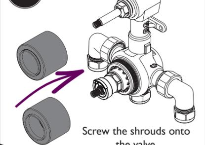
Screw the shrouds onto the valve.
