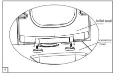
4. Close the hinge cap and re-attach the seat into hinge.
