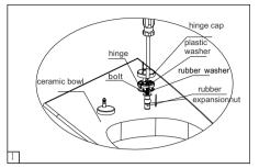
1. Insert rubber expansion nut into bowl bolt holes, then install hinge, plastic washer and bolt into hinge holes. Using screwdriver to tighten the bolt into rubber expansion nuts and close the hinge cap.
