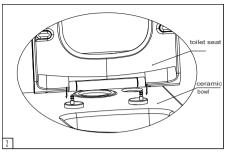
2. Attach the seat cover into hinge bar as per drawing.
