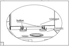
3. Slightly press the hinge cap, lift the seat cover to separate from hinge.
