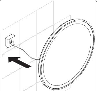
Using the brackets on the reverse of the mirror, offer up the mirror to the desired position. Ensure the mirror power cable is within reach of the connection to the power supply box (not supplied) from the electrical mains.
