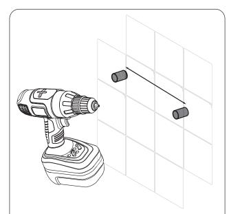
Using a suitable drill bit, drill holes in the marked positions to fit the wall plugs and screws provided. If drilling through tile, use a ceramic drill bit. NB For plasterboard walls, specialist fixings should be purchased
