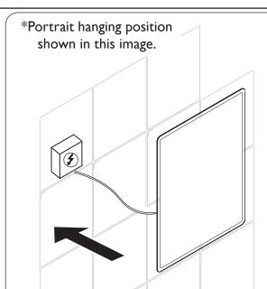
Using the brackets on the reverse of the mirror, offer up the mirror to the desired position. Ensure the mirror power cable is within reach of the connection to the power supply box (not supplied) from the electrical mains.
