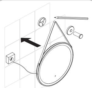
Fix the leather strap to the mirror, using the screws provided. Using the hanging hook and wall bracket, offer up to the desired position and carefully mark the holes using a pencil. Ensure the mirror power cable is within reach of the connection to the power supply box (not supplied) from the electrical mains.
