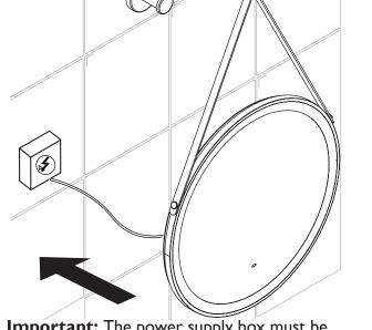
Important: The power supply box must be permanently connected to the fixed wiring of the mains supply using the supplied power cable. Hang the mirror onto the fixings and ensure it is safe and secure.
