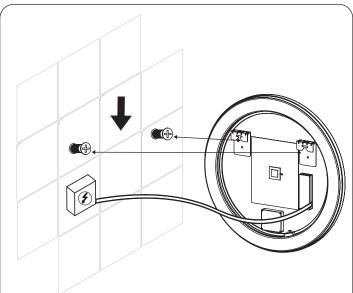
**Important:** The power supply box must be permanently connected to the fixed wiring of the mains supply using the supplied power cable and power supply box (not supplied).
