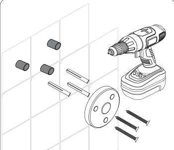
Using a suitable drill bit, drill holes in the marked positions to fit the wall plugs and screws provided. If drilling through tile, use a ceramic drill bit. NB For plasterboard walls, specialist fixings should be purchased. Screw the chrome wall bracket into place
