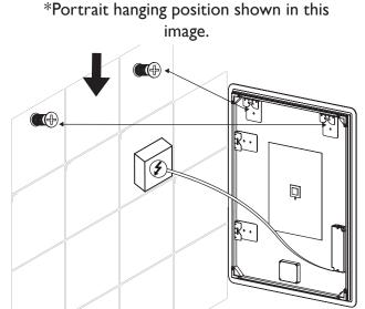
**Important:** The power supply box must be permanently connected to the fixed wiring of the mains supply using the supplied power cable and power supply box (not supplied).
