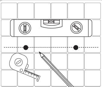
Carefully mark the fixing points using a tape measure, a pencil and spirit level, using the dimensions given on page 6 and the brackets on the reverse of the mirror as a guide. Please ensure that all marked mounting points accurately match up with the fixing points on the mirror
