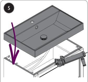
Ensure the basin will evenly align on top of the unit when pushed up to the wall. Remove the basin. Apply a bead of silicon sealant to the top left and right side edges of the unit only, before the basin is finally positioned.
