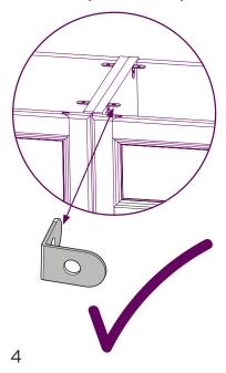
If you are fitting the Claverton basin, you will need to cut a notch like this either side of the worktop, to alllow for the basin to sit correctly next to the worktop.
