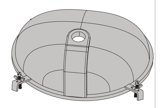
Fixing Kit (4 x Screws, 4 x Wingnuts & Washers, 4 x Brackets)
