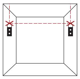
4. Drill the appropriate sized hole for your wall plug and screw and fit your hooks accordingly.
