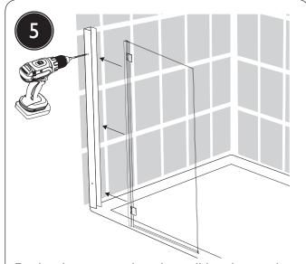
Fit the shower panel to the wall bracket so that the sealing strip on the base rests enough to create a seal but light enough to move. Using the drill bit provided drill two holes. Place the provided cover housing over the holes and secure using screws provided. Use the provided caps to hide the screw heads.
