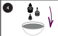
Remove any O-rings and soak all components in de-scaler. Rinse throroughly in clean water. Examine all seals and replace if needed. Use a WRAS approved silicon based grease on all seals.
