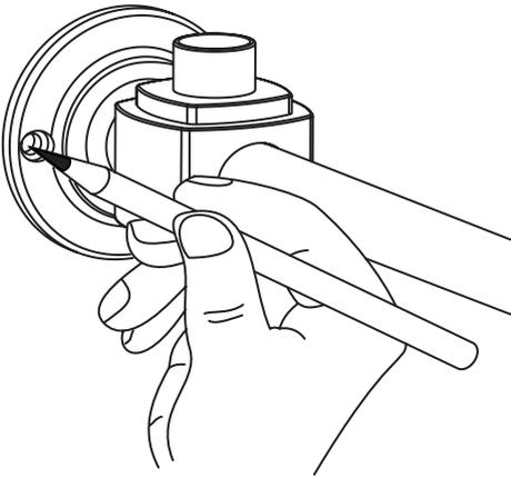
Locate the washstand on the newly installed Foot Stops and mark the location for the holes in the wall by using the washstand holes as the template. Ensure the washstand is level using a spirit level. Move the wash stand out of the way and drill suitable holes.
