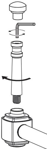
With the washstand in the correct position, fix the chrome columns to the stand. Using the 5mm hexagonal key to tighten and secure the columns. Add the Basin rests to the top of the chrome columns.
