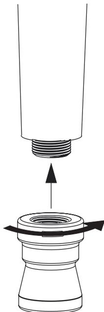
Attach the washstand feet to the base of the leg assemblies.
