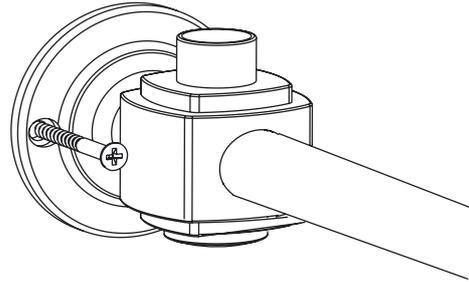
Secure the wash stand to the wall using suitable screws and wall plugs, depending on the wall type.
