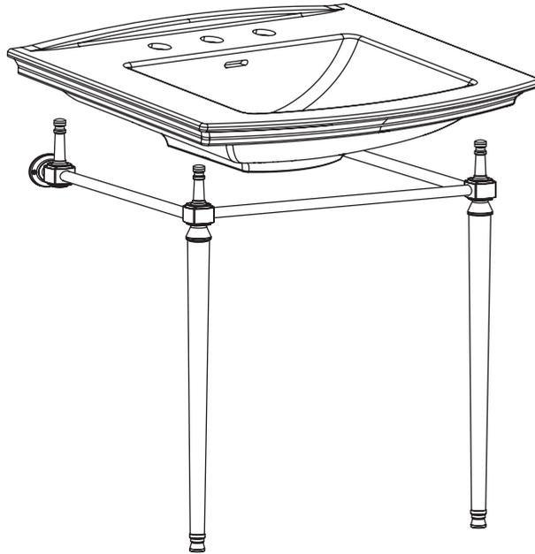
Locate the basin on the four chrome columns. If the product is supplied with inserts as seen in section 10, bear in mind that these need to be installed before levelling the basin.
