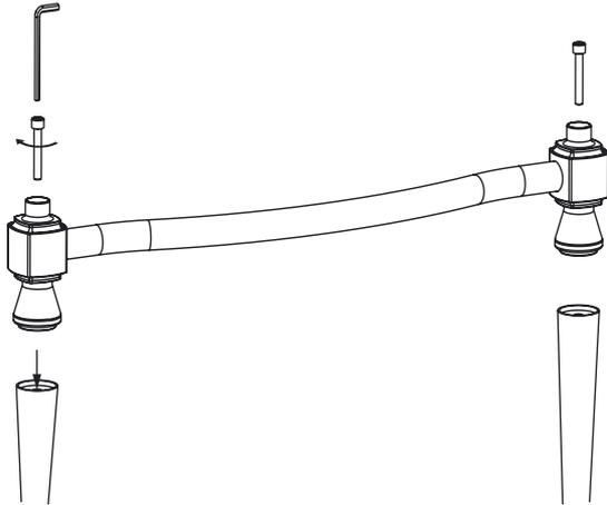
Attach both leg assemblies to the bottom of the front pole assemblies by using the M6 (35mm) hex bolt to secure the parts together.
