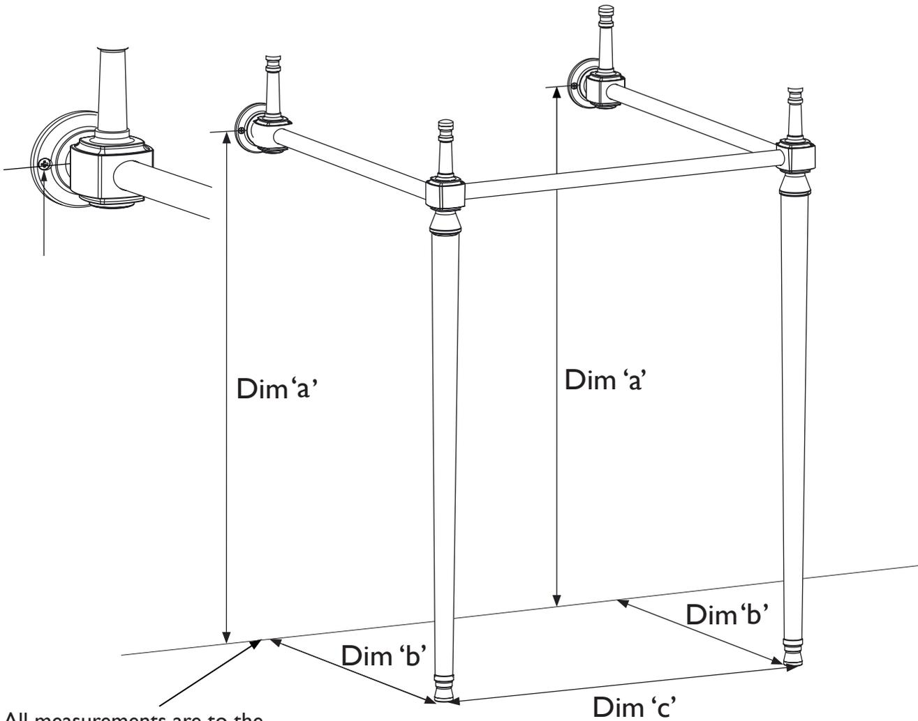
All measurements are to the centre of the legs, Dimension 'b' is measured to the wall and not the skirting board.
