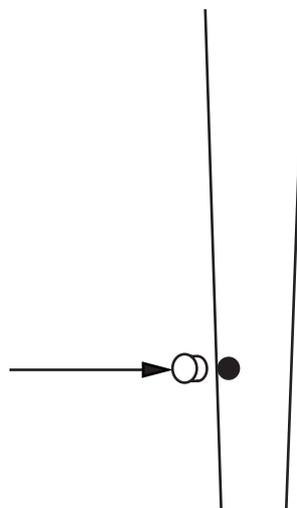
If the glass shelf is not going to be installed then use the 6 blanking plugs to cover the holes on the washstand.
