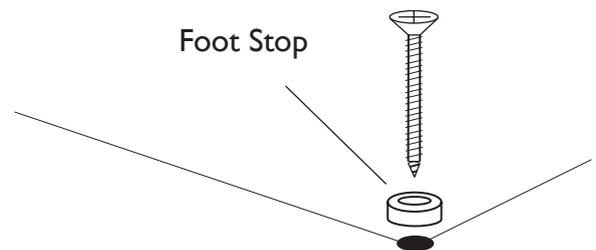
Using the dimensions (b & c) based on your washstand (page 5), accurately measure, mark and drill the holes in the floor for the foot stops and secure them down using the screws and suitable fixings for floor type.
