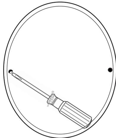
Mount the mirror using the spacers and screws supplied (if applicable to the wall. **DO NOT OVERTIGHTEN OR YOU RISK BREAKING THE MIRROR.** Check the mirror for security.
