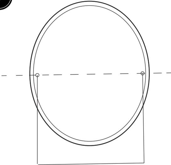
Offer the mirror up to the desired position. Measure the distance between the holes on the mirror.
