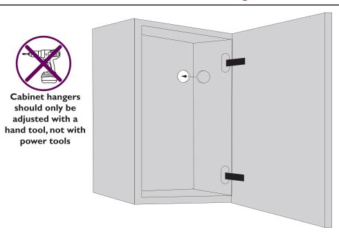
Turn the top adjustment screw to adjust the unit from front to back. Allows unit to tilt forwards or backwards from the wall.
