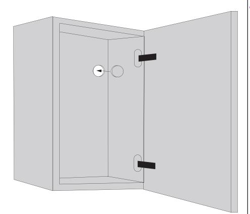
Locate the wall units in position and mark up where they will be secured to the wall.
