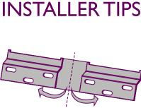
The wall units are supplied with suspension fittings that are pre-fitted to the back of the unit. The wall hanging brackets will be supplied joined together, you will need to seperate them by snapping them apart. Hold eitherside of bracket and gently snap them apart.
