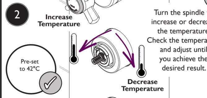
Turn the spindle to increase or decrease the temperature. Check the temperature and adjust until you achieve the desired result.
