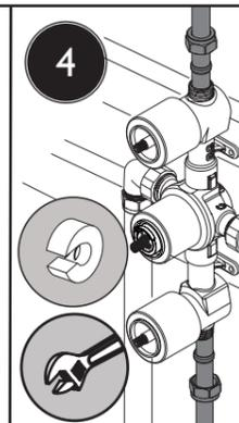
Plumb your chosen outlets into the valve. Turn on the water supply and check the valve for any leaks.
