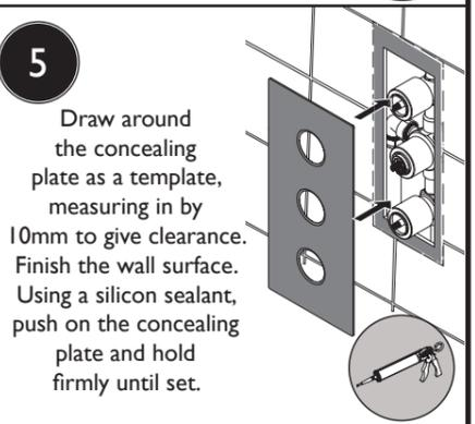
Draw around the concealing plate as a template, measuring in by 10mm to give clearance. Finish the wall surface. Using a silicon sealant, push on the concealing plate and hold firmly until set.
