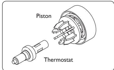
4. Grease the seals with a silicon greas and carefully refit.
