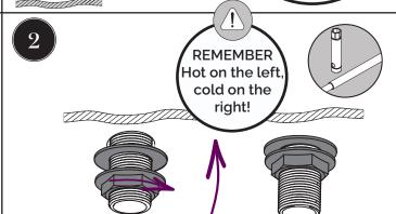
Secure the taps to the basin/bath by using the washer and metal backnut below the basin. Ensure the washer is correctly positioned between the backnuts and the basin/bath.
