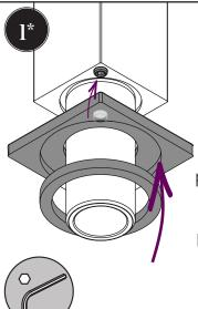
Some plinths will need to be aligned with a pre-attached grub screw.
