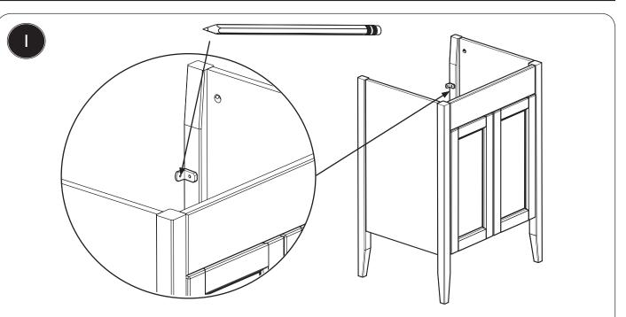
This unit may be fixed to the wall using angled brackets (Not Supplied). Hold the cabinet in the required location and with a pencil, mark the wall and unit through the holes in the angled brackets. It is best to install the angled brackets on the inside of the freestanding furniture.
