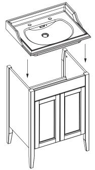
Locate the basin so it is evenly flush with the edges and filmly against the rear wall. Fasten basin to the wall using screws (not supplied) or bolts (supplied). The holes for these can be seen on the rear of the basin.
