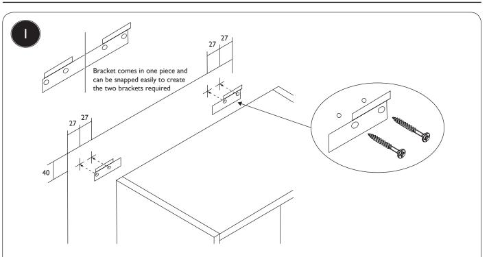
Wall Units are hung on adjustable wall hanging brackets. The brackets are supplied with wall hanging plates, which should be secured to the wall with suitable wall fixings.
