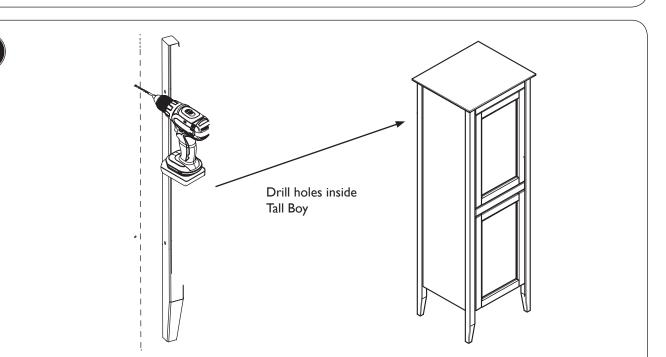
Remove the tall boy cabinet and drill holes of the appropriate size to accept the necessary screws or wall plugs used to secure. Lift the tall boy cabinet back into position and screw to the wall.
