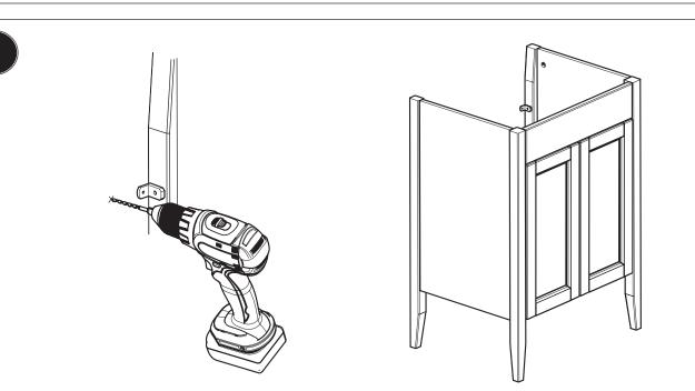
Remove the cabinet and drill holes of the appropriate size to accept the necessary screws or wall plugs used to secure. Lift the cabinet back into position and screw to the wall.
