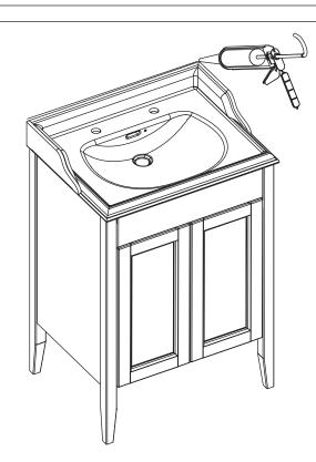
Use silicon sealant where necessary to ensure the basin edges are sealed and water tight to the furniture and wall. Refer to any instructions provided with handles when fitting to the doors.
