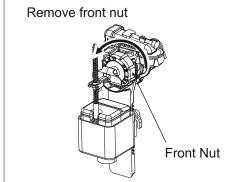
Remove filter from valve, wash with clean water and re-assemble. Ensure the float chamber is in position shown. If necessary press tabs
