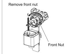
Remove filter from valve, wash with clean water and re-assemble. Ensure the float chamber is in position shown. If necessary press tabs to reposition
