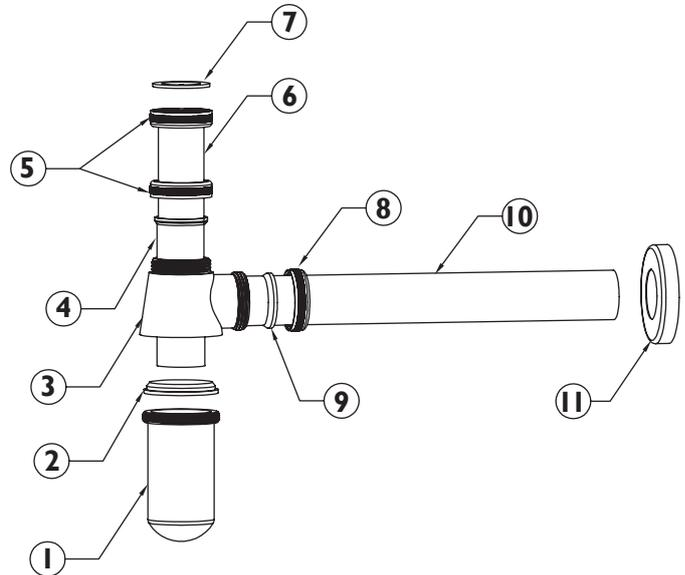
1. Screw the waste trap (1) to the waste body (3), ensuring the rubber washer (2) is in place.
