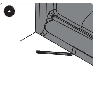
Mark the floor fixing holes. Check whether your pan is supplied with screws or foot fixings. Where no fixings are supplied, make sure to use suitable screws for your floor type.
