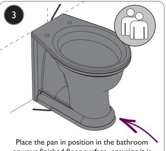
Place the pan in position in the bathroom on your finished floor surface, ensuring it is level and its back is in full contact with the wall. Using a pencil, make a horizontal line along the back edge of the pan and the outer edge of the base.
