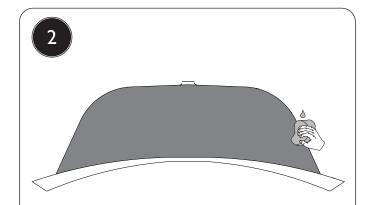
Check the outside surface for any damage and that it is clean and free of any impurities e.g. dirt, dust, grease etc. If cleaning is required, thoroughly clean and degrease the surface with Acetone or alcohol. Make sure you allow this to dry before you begin painting.
