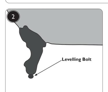
Carefully turn the bath back to its upright position. Using a spirit level, check the top of the bath is level. If necessary, use the levelling bolts on each foot to remove rocking and make the bath level.
