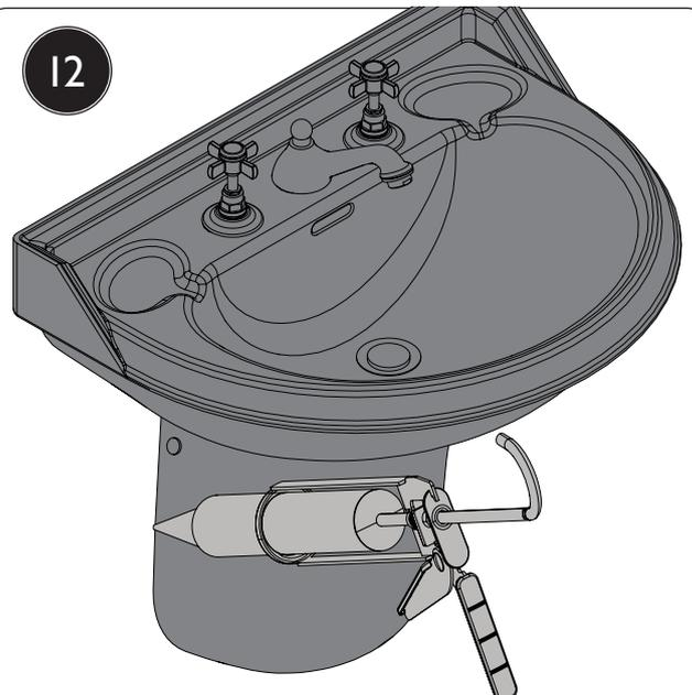
Use a suitable silicon sealant around the back of the basin and around the edge of the pedestal to keep watertight.
