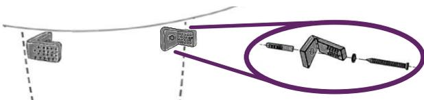
Refer to the instructions on the fixings pack to install the fixing brackets.
