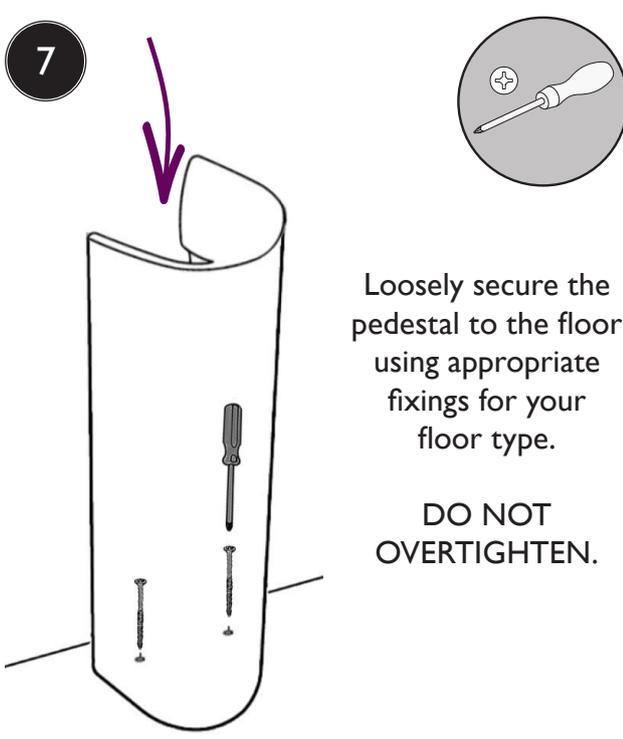
Loosely secure the pedestal to the floor using appropriate fixings for your floor type.
