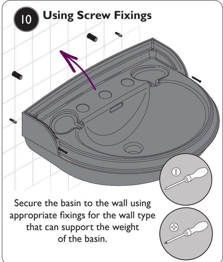
Secure the basin to the wall using appropriate fixings for the wall type that can support the weight of the basin.
