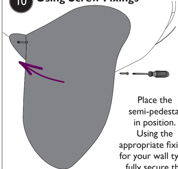
Place the semi-pedestal in position. Using the appropriate fixings for your wall type, fully secure the pedestal to the wall.
