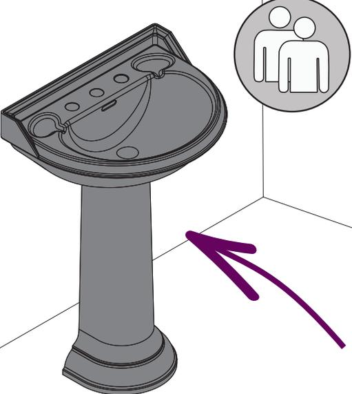
Place the basin on the pedestal and move to the required position in your bathroom. Ensure the basin is correctly positioned on the pedestal, the basin and pedestal are level, and the back of the basin is in full contact with the wall.
