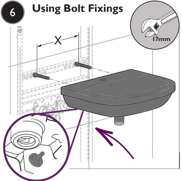
Locate the basin on to the threaded bolts. Ensure the basin is level and secure with nuts and washers.
