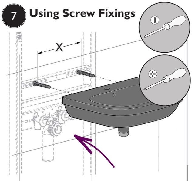
Locate the basin on to the threaded bolts. Ensure the basin is level and secure the basin to the wall using suitable fixings to support the weight of the basin.
