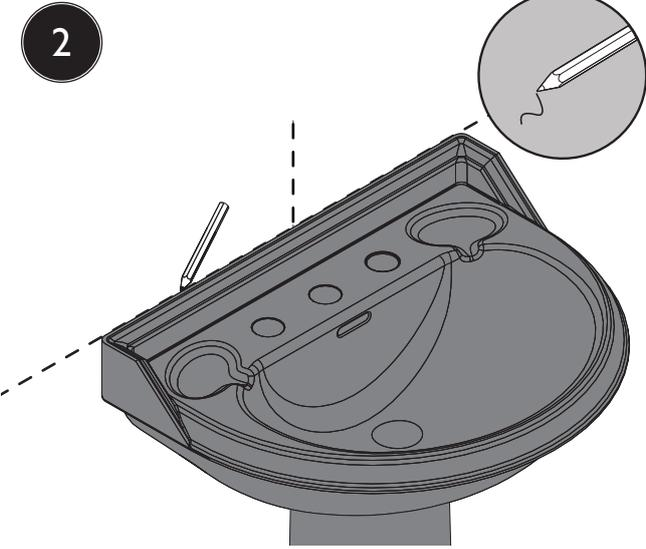
Mark the centre of the basin on the wall. Make a horizontal line along the back edge of the basin and trace along the outer edge of the pedestal. Mark the position of the bolt/screw holes on the basin and pedestal.
