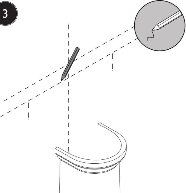
Remove the basin. Draw a horizontal line through the bolt/screw holes and carry the centre line down until it meets the bolt/screw holes on the basin.
