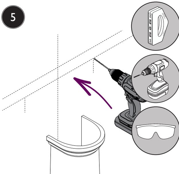
Drill each fixing hole, taking into account the screws and wall plugs (not supplied). Install the threaded bolts if bolt fixings are supplied. If necessary, also drill the holes required for any pipework.
