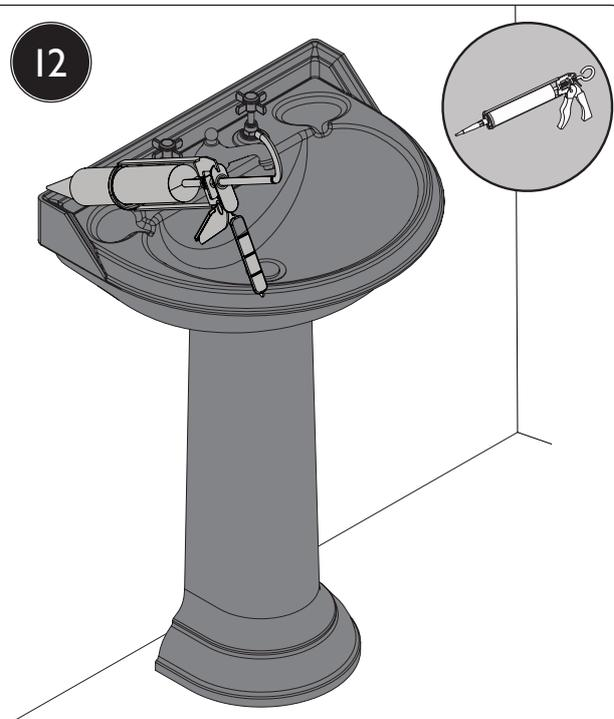
Use a suitable silicon sealant around the back of the basin to keep watertight.
