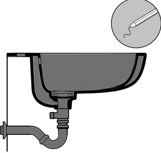
Refer to your tap and waste instructions to install these on to the basin, including the waste trap. Place the basin back on to the pedestal and mark on the wall the locations of the waste pipework and the hot and cold connections.
