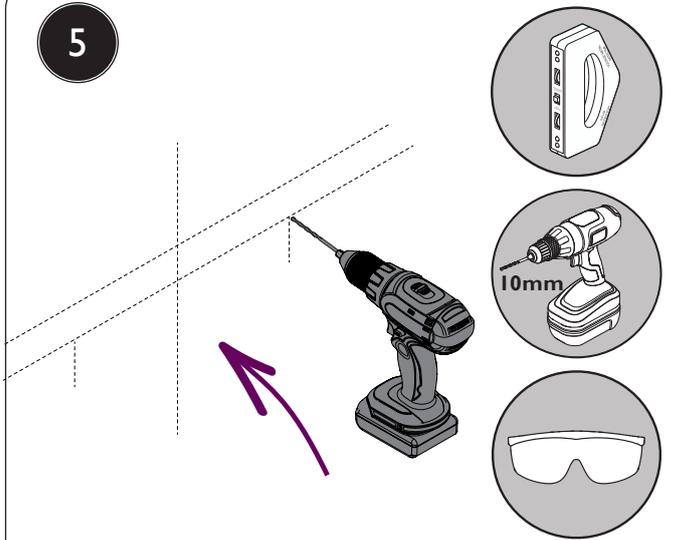
Drill each fixing hole for the basin and pedestal, taking into account the screws and wall plugs (not supplied). Install the threaded bolts if bolt fixings are supplied. If necessary, also drill the holes required for any pipework.
