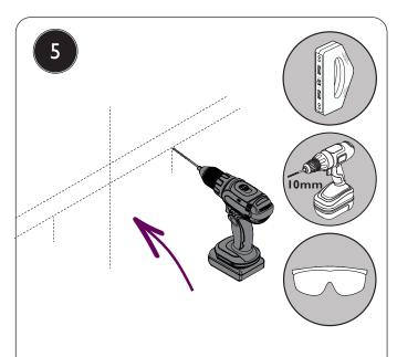
Drill each fixing hole for the basin and pedestal, taking into account the screws and wall plugs (not supplied). Install the threaded bolts if bolt fixings are supplied. If necessary, also drill the holes required for any pipework.
