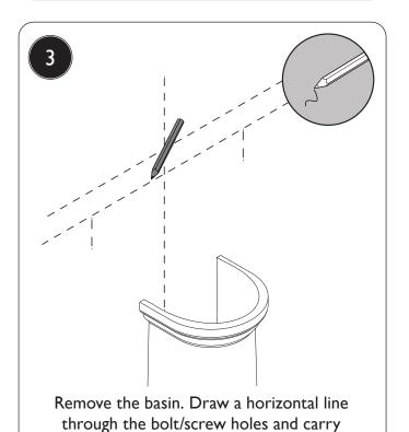
the centre line down until it meets the bolt/screw holes on the basin.
