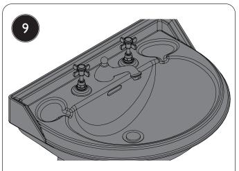
Turn on the water supply at the isolation valve and check for leaks.
