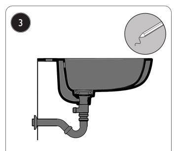
Refer to your tap and waste instructions to install these on to the basin, including the waste trap. Place the basin back in its position and mark on the wall the locations of the waste pipework and the hot and cold connections.
