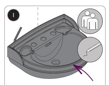
Place the basin in the desired location in your bathroom. Ensure the basin is level, and the back of the basin is in full contact with the wall. Using a pencil, mark the centre of the basin on its tap ledge, extend this line up where it meets the wall. Make a horizontal line along the back edge of the basin and trace along the bottom of the basin.
