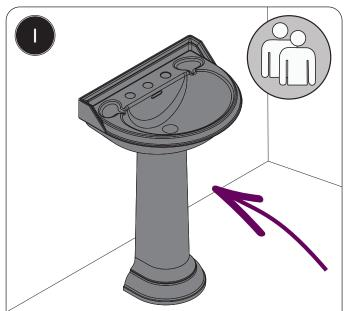
Place the basin on the pedestal and move to the required position in your bathroom. Ensure the basin is correctly positioned on the pedestal, the basin and pedestal are level, and the back of the basin is in full contact with the wall.
