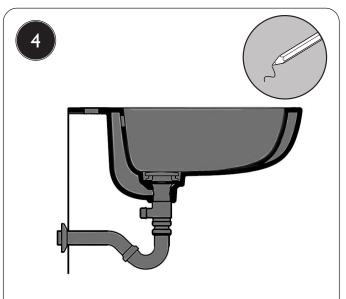
Refer to your tap and waste instructions to install these on to the basin, including the waste trap. Place the basin back on to the pedestal and mark on the wall the locations of the waste pipework and the hot and cold connections.
