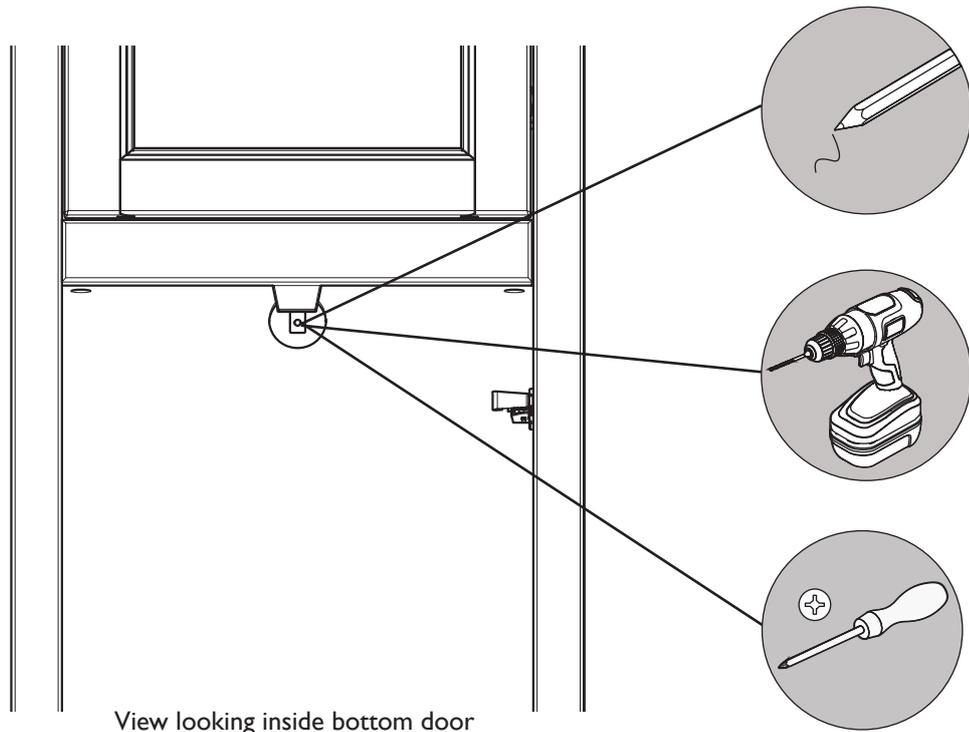
Mark the required hole using the bracket hole as a template. Drill a suitable hole for the wall fixings used (not supplied). Attach the bracket to the wall.
