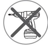
Cabinet hangers should only be adjusted with a hand tool and not a power tool
