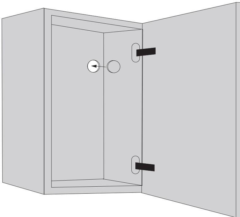
Once adjustment has been completed, the covering cap can be pressed on, to conceal the hole.
