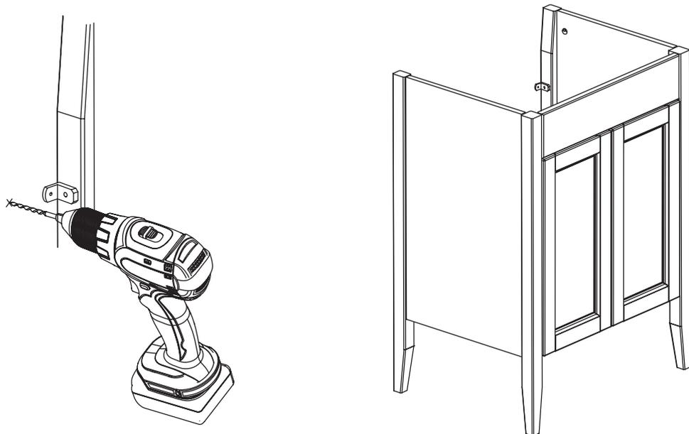
Remove the cabinet and drill holes of the appropriate size to accept the necessary screws or wall plugs used to secure. Lift the cabinet back into position and screw to the wall.
