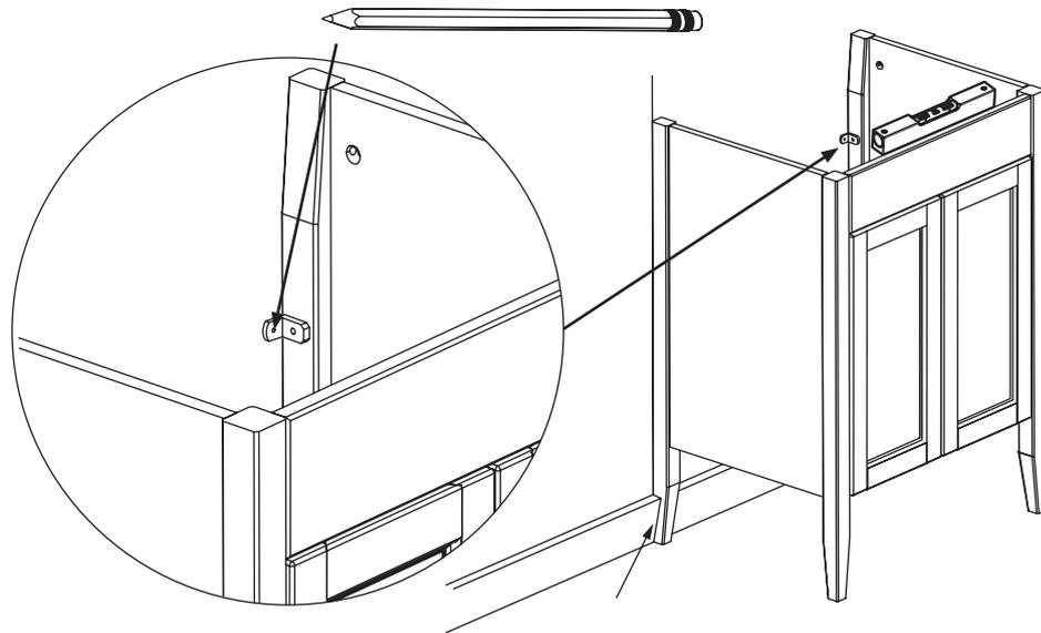
We recommend that you secure the unit to the wall using angled brackets (not supplied). Position the cabinet in your required location checking the alignment with a spirit level and mark the wall through the holes in the angled brackets. Make sure you removed required skirting boards before fixing. It is best to install the angled brackets on the inside of the freestanding furniture.
