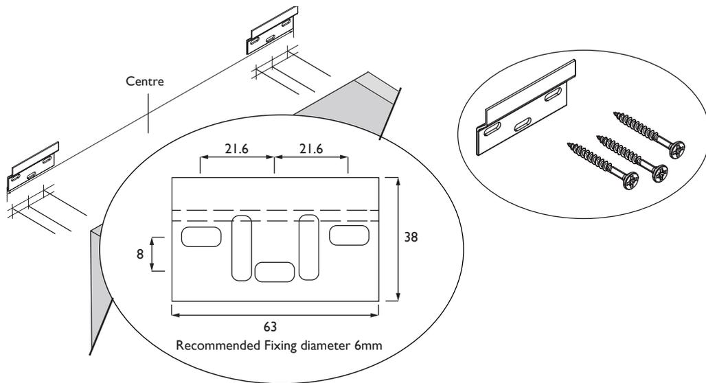
Determine favoured position of cabinet and mark a vertical centre point on the wall. Measure the span of the pre-fitted brackets and transfer measurement to wall measurement out from centre point to give a central position for the cabinet. Fit the wall plates using appropriate fixings (not supplied) using a long spirit level to make sure levelling is accurate. Plates should be no more wide apart than the spanned measurement of the wall hanging brackets.
