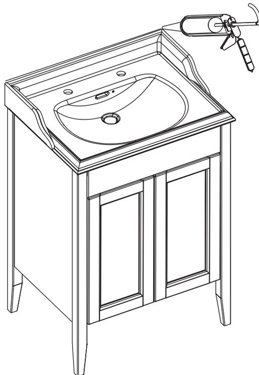
Once basin is fixed to the wall, run a bead of silicon around the joint between the basin and the vanity unit, this will ensure the furniture is sealed from water. Handles should be fitted by referring to accompanying instructions.
